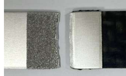
Tensile shear strength: 20 MPa
